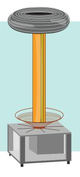
**CONCEPT** A Tesla coil is a device for creating high voltages. Voltage is a way to measure how much energy an electric charge has. Tesla coils can create voltages over 1 million volts. Typically, such high voltages are dangerous, but the Tesla coil handles high frequency electricity. This means the coil turns on and off so quickly that electricity flows on the outside of skin instead of through the body.
